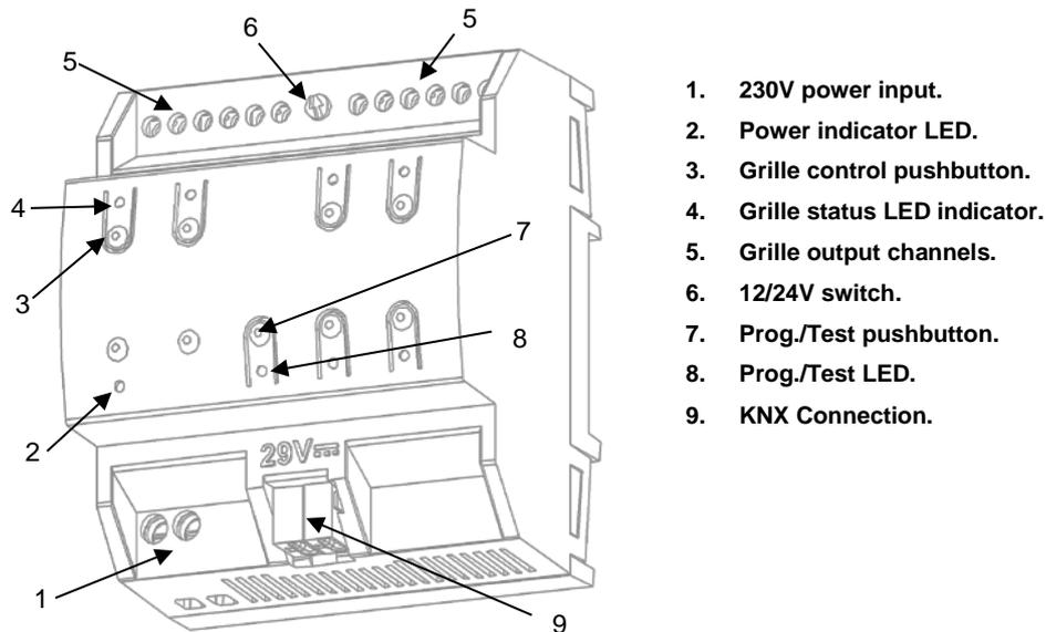
Figure 2. Element diagram (ZoningBOX 6)
