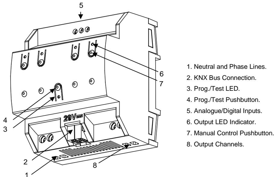
Figure 3 DIMinBOX 2CH - Element Diagram.
