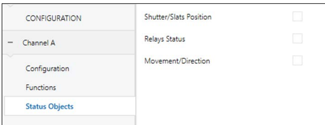
Figure 3 Shutter Channel – Status Objects.
