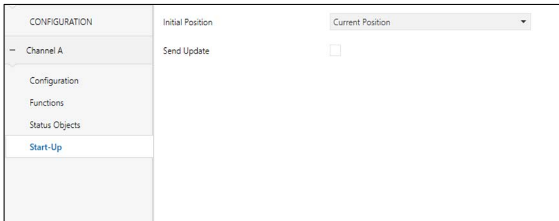
Figure 8 Shutter Channel - Start-Up.
