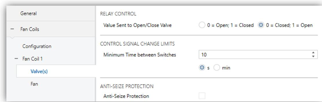
Figure 5. Fan Coil – Binary Valve – Fan-Oriented Control.
