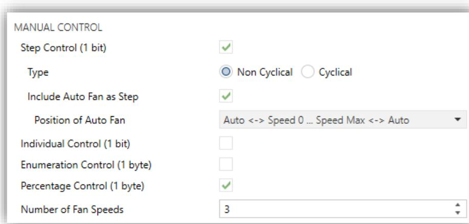
Figure 11. Fan Coil – Manual Fan Control.
