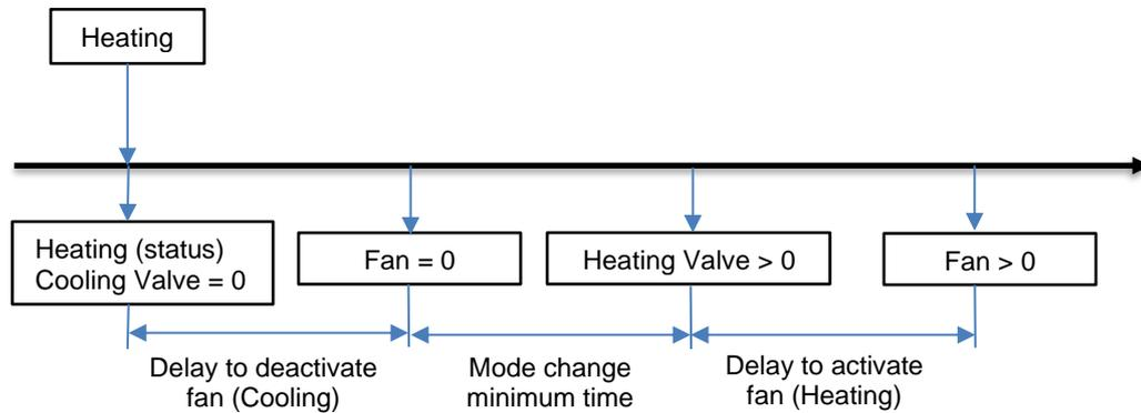
Figure 9. Delay for fan activation/deactivation.
