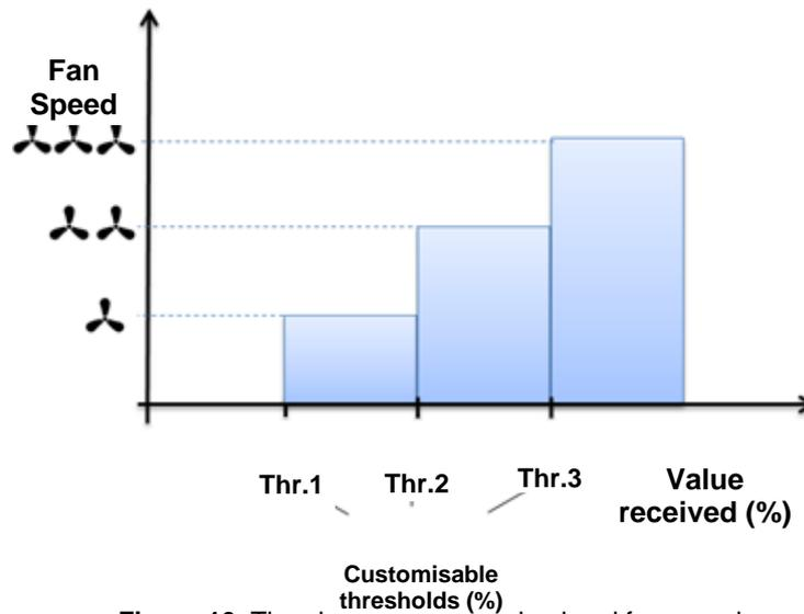
Besides, a **hysteresis** can be configured to avoid continuous relays switching when the control signal oscillates around the parameterised thresholds. This way, when the control signal is greater than the configured threshold plus the hysteresis, the system will switch to the immediately upper speed; and to the immediately lower speed when the control signal is lower than the threshold minus the hysteresis.
