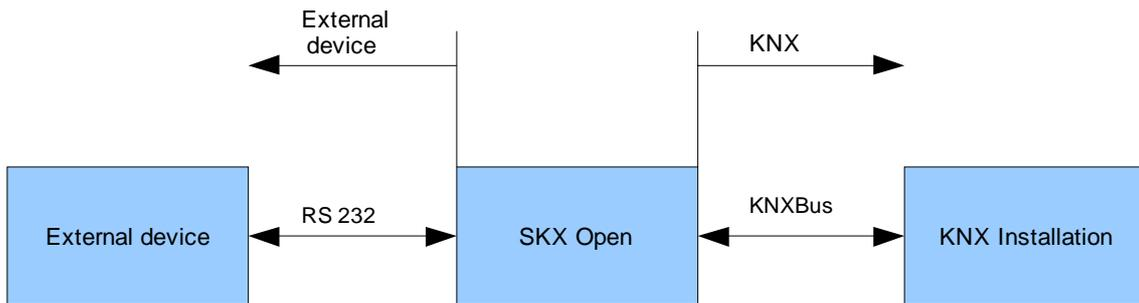
**Figure 1. SKX Open Bidirectional Communication**
