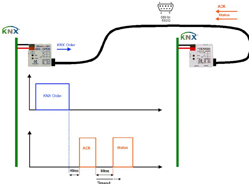
Figure 6. Example with SKX Open and SKX Open
