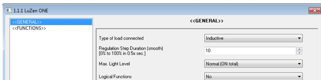
Figure 3.2. Parameterization screen by default
