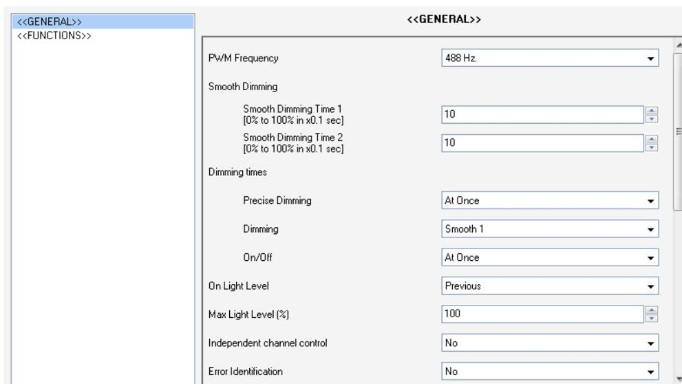
Figure 5. Parameterisation screen by default
