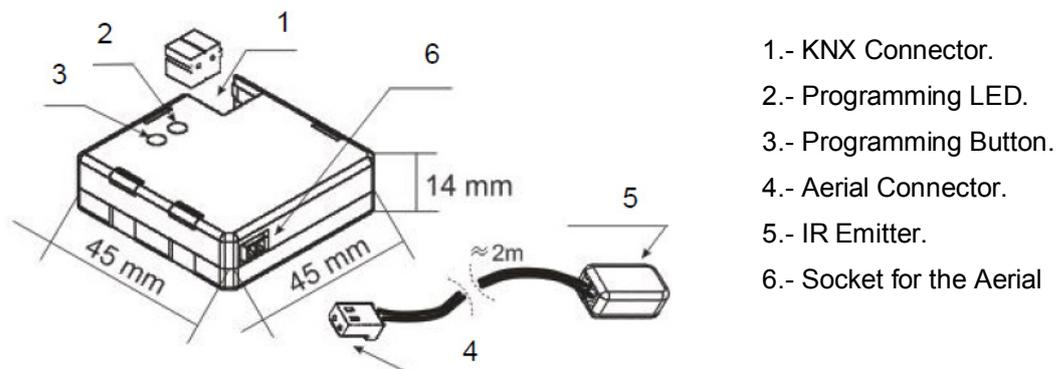
Figure 2. IRSC Element diagram
