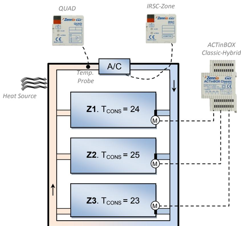
Under these circumstances, if the “External Temperature Returned” parameter is found to be disabled, IRSC Zone analyses the temperature setpoints of zones Z1 and Z2 (since Z3 has been switched off):
