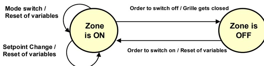
Figure 12. "Zone ON" / "Zone OFF" state diagram
