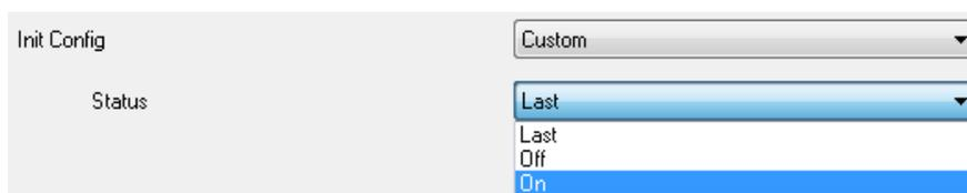
**Last:** Fan Coil will recover the status before the voltage supply drop.
