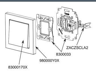
Figure 1. Single push button switch
