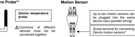
\* In case of using ZN1IO-DETEC-P sensor, its micro switch number 2 must be in Type B position.
