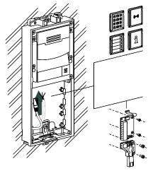
Fix the blind panel (or additional modules that remain in sight) with the supplied screws and put the labels with captions next to the buttons.
