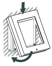
6 Fix the frame by using the supplied Allen key.
