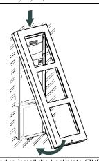
6 Fix the frame using by the supplied Allen key.
