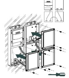
Place the frames and fix them by using the supplied Allen key.
