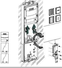
4 Fix the blind panel and additional modules that remain in sight with supplied screws and put the labels with captions next to the buttons.
