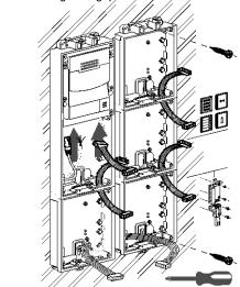
5 Interconnect the additional modules with the bus as indicated in the schema and then fix the additional modules with the screws.
