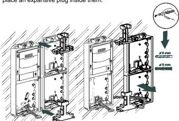
**4** Fix the right assembly to the wall with screws. Make the connections of the basic unit and prepare the additional modules. Pass the bus cable through the gaps.
