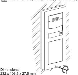
Note: it is recommended to install the backplate (ZVP-BPLA2) if the wall surface irregularity is greater than 0.5mm.
