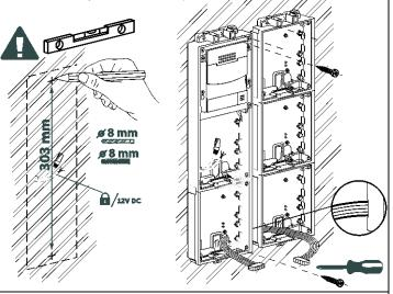
3 Place the right assembly on the wall by using the T-shape parts. Mark the position of the holes, drill them and afterwards place expansive plugs inside.
