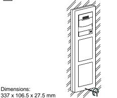
Note: it is recommended to install the backplate (ZVP-BPLA3) if the wall surface irregularity is greater than 0.5mm.
