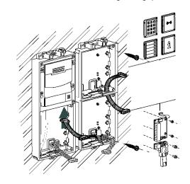
**5** Interconnect the additional modules with the bus as indicated in the schema and then fix the additional modules with screws.
