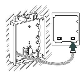
4 Fix the additional module with the supplied screws.
