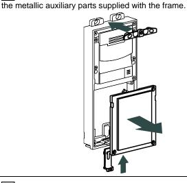
Place the basic unit correctly levelled on the wall and drill two holes for the expanding plugs. Recover the cables and fix the module with the screws (included).
