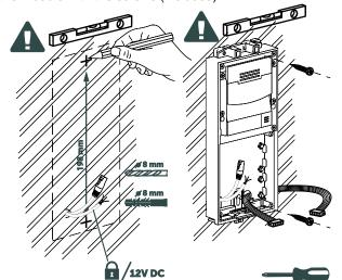
Place the right assembly on the wall by using the T-shape parts. Mark the position of the holes, drill them and afterwards place an expansive plug inside them.
