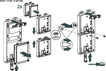
Place the left assembly correctly levelled on the wall and drill two holes for the expansive plugs. Recover the cables and fix the module with the screws (included).
