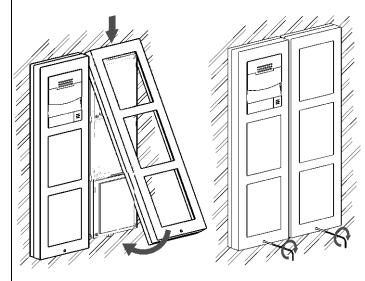
Note: it is recommended to install the backplate (ZVP-BP2W3H, ZVP- BP3W3H) if the wall surface irregularity is greater than 0.5mm.
