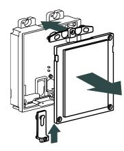
Place the additional module enclosure correctly levelled on the wall and drill two holes for the expanding plugs. Recover the cables and fix the enclosure with the screws (included).
