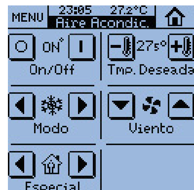
Climate Page set for Air Conditioning control with Thermostat included
