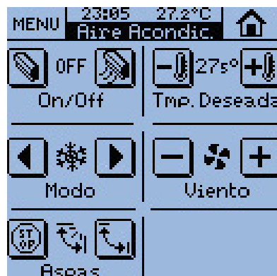
Climate Page set for Air Conditioning Control
